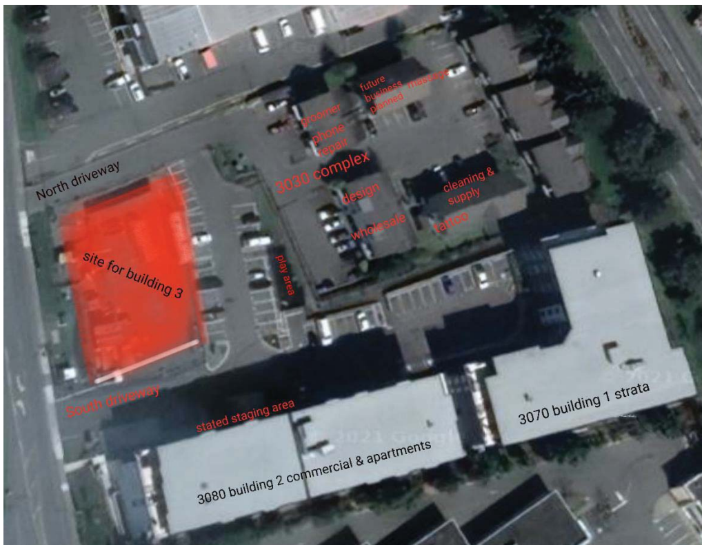
7. A view of the site from Google Earth. There is nowhere to stage construction without impeding access since the proposed residential block would take the entire footprint of the site. There is nowhere for tradespeople or workers to park without taking the parking of neighbourhood businesses meant for their customers. You can also note the lack of any open areas. The “Play area” is the very small, dark spot near the centre and is comprised of two benches and cigarette butt cans, some rubber matting and a small strip of grass. It is about three car lengths.
